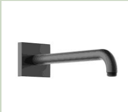
53088 130402 WALL MOUNTED SHOWER ARM G ½", W80 X H80 X D450 mm Opportunity of alignment on the wall (90° ± 2°) and wall connection (90° ± 5°)
