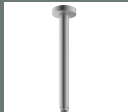
51689 050300 CEILING MTD SHOWER ARM G1/2", W80 x H300 x D80 mm Opportunity of alignment on the ceiling (90° ± 2°) and ceiling connection (90° ± 5°) Also available in H100mm
