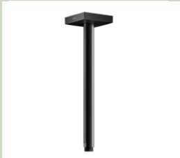
53089 130302 CEILING MTD SHOWER ARM G1/2", W80 X H300 X D80 mm Opportunity of alignment on the ceiling (90° ± 2°) and ceiling connection (90° ± 5°) Also available in H100mm
